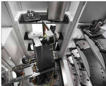
HS flex with two pallet storage modules and a setup station, adapted to a C 42 U machining centre.
