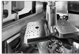
Double gripper for 2 x 150 kg
